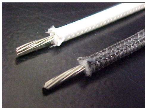
SEW-2 – 600V, 200°C (392°F) Silicon / Rubber / Glass
